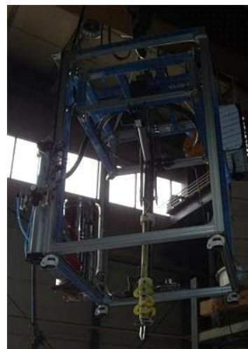
Fig. 1. Spent Resin Sampler for in-station storage tank within Wolsong a NPP.
