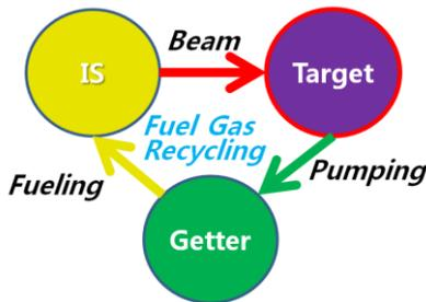
Fig. 3. D/T gas recycles in a portable neutron generator.
