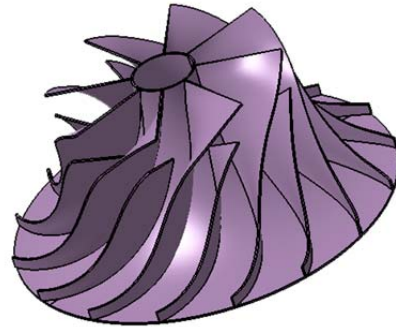
Fig. 4. 3D impeller model of iSFR S-CO 2 Compressor
