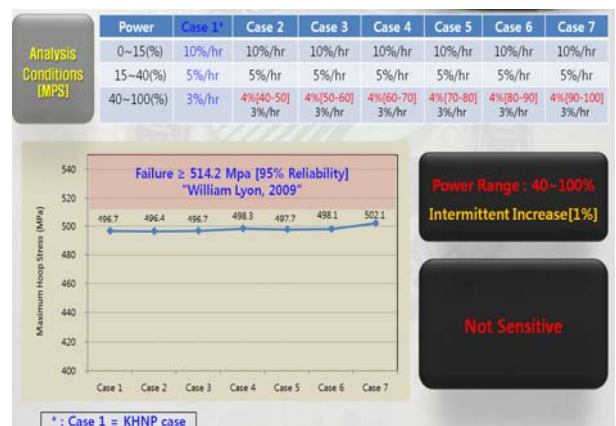
Figure 3-5. Maximum Hoop stress about the intermittent increase(1%) of startup ramp rate in 40~90% power range
