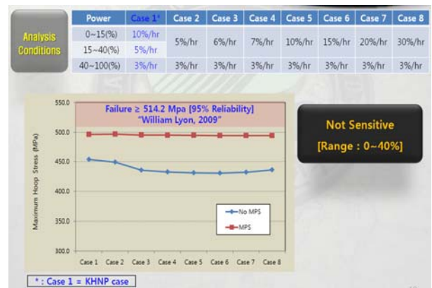
Figure 3-4. Maximum Hoop stress about the change of startup ramp rate in 0~40% power range
