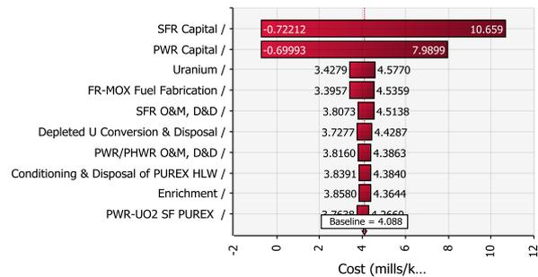
Fig. 5. Value tornado diagrams for the variation of LCT gap between Scenario 1 and 4 for each fuel cycle step.
