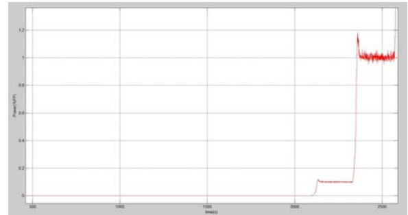
Fig. 5. Power control performance around 0.1% and 1% of power
