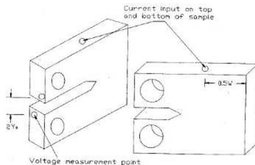
Fig. 2 Input current and voltage lead locations
