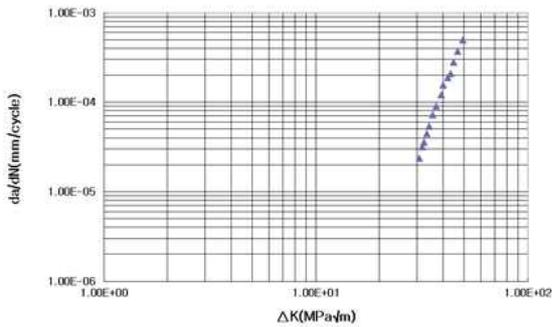
Fig. 5 da/dN- $\Delta K$  at 500°C
