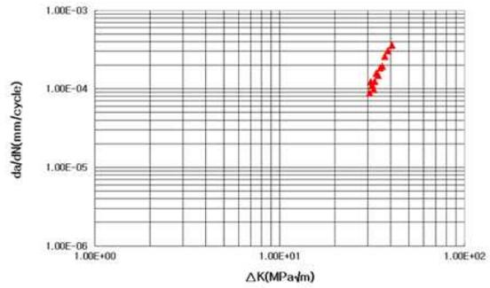
Fig. 7 da/dN- $\Delta K$  at 600°C
