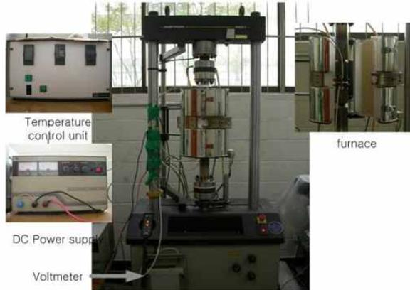
Fig. 4 High temperature creep-fatigue crack growth test facility
