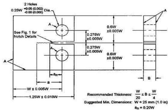
Fig. 1 CT specimen for the creep-fatigue crack growth test
