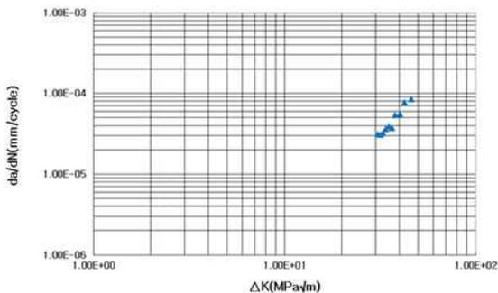
Fig. 6 da/dN- $\Delta K$  at 550°C
