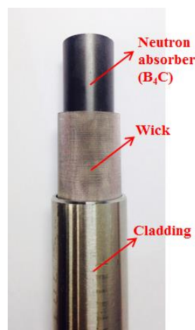
Fig. 1. Composition of hybrid control rod.
