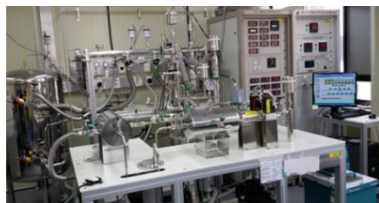
Fig. 7. A DU bed system for storing/supplying hydrogen isotopes and simulating tritium inventory.
