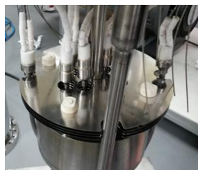
Fig.3. Wiring of thermal shield.
