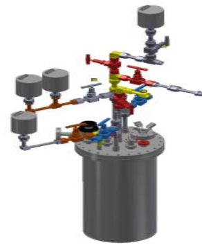
Fig.1. Schematic models of a DU bed.
