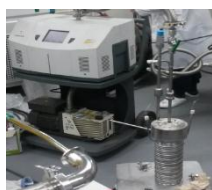
Fig.6. Leak and pressure test of a primary vessel.
