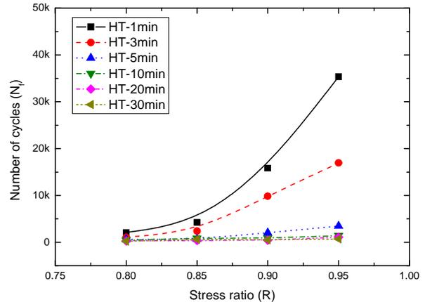
Fig. 3. Variations of number of cycles as a function of stress ratio at each hold time.
