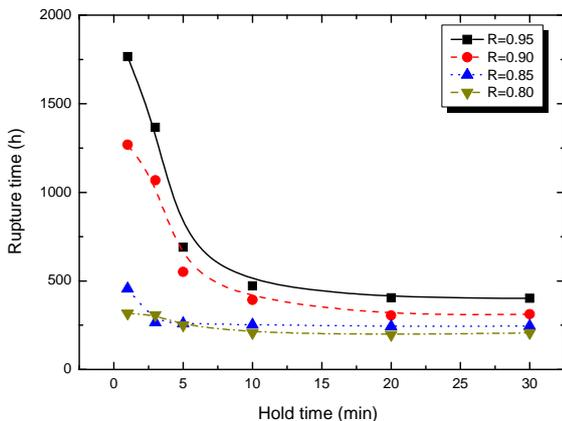
Fig. 1. Variations of the cyclic creep rupture time with the hold times at each stress ratio.
