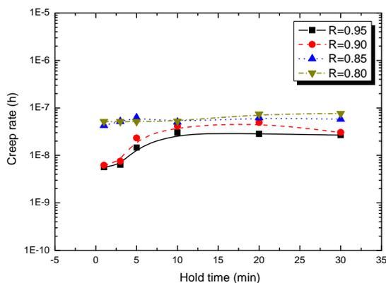
Fig. 2. Variations of the creep rate with the hold times at each stress ratio.
