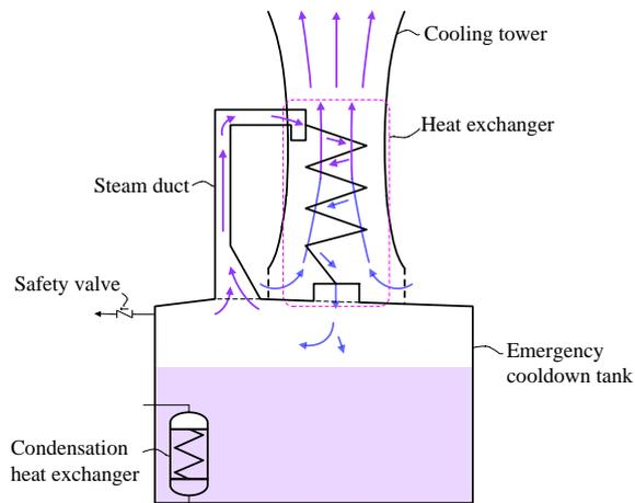
Fig. 1. Schematic of air natural convective cooling system of emergency cooldown tank.
