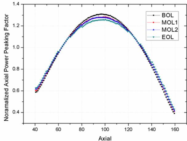
Fig. 9. Normalized Axial Power Distribution
