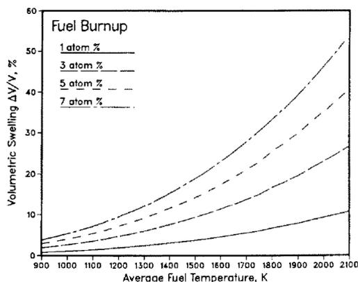
Fig. 3. Predicted UN fuel swelling against volume-averaged fuel temperature [6]
