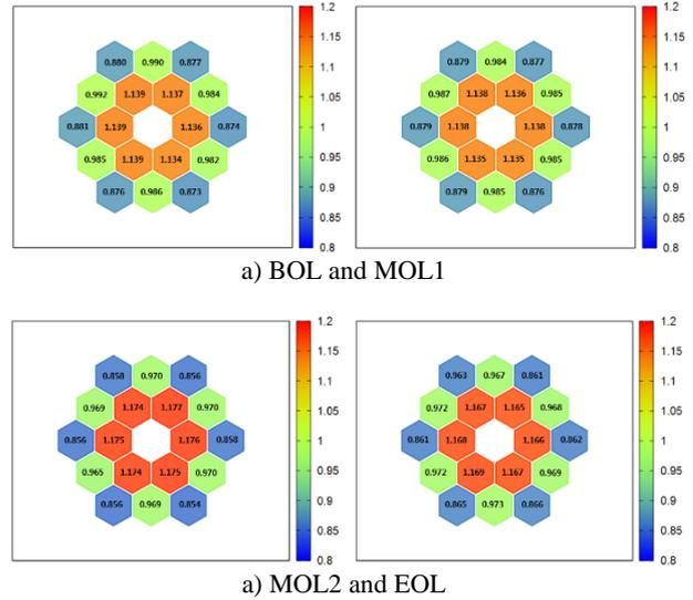
Fig. 8. Normalized Radial Power Distribution
