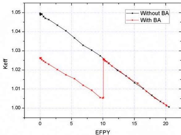
Fig. 7. Depletion results of with and without BA
