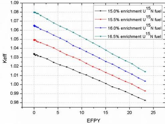
Fig. 6. Depletion results with different enriched U<sup>15</sup>N fuel
