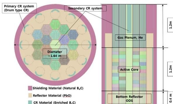
Fig. 4. Radial and axial configurations of MMR core
