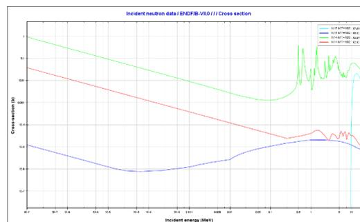
Fig. 2. Comparison of <sup>14</sup>N and <sup>15</sup>N (n,γ) and (n,p) cross section [5]
