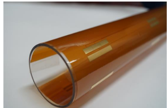
Fig. 2. Shape of three-ring conductance meter on FPCB
