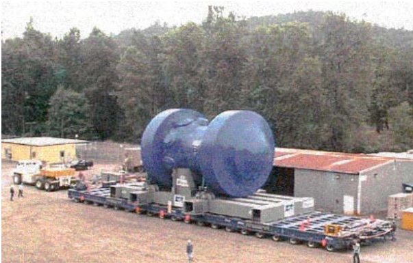
Fig. 2. Vessel package from Trojan NPP transported to disposal site by barge[8].
