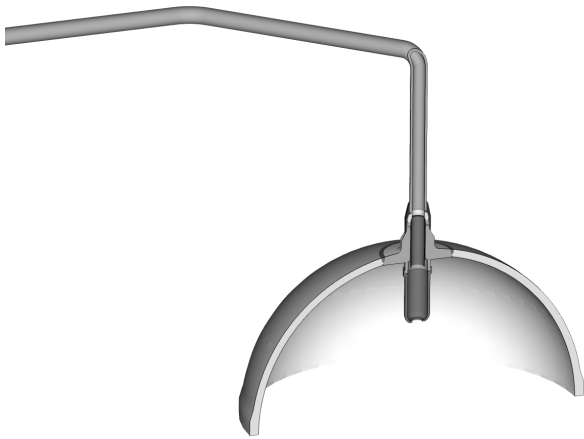
Fig. 1. Configuration of Spray Line Pipe and Nozzle attached on the Pressurizer
