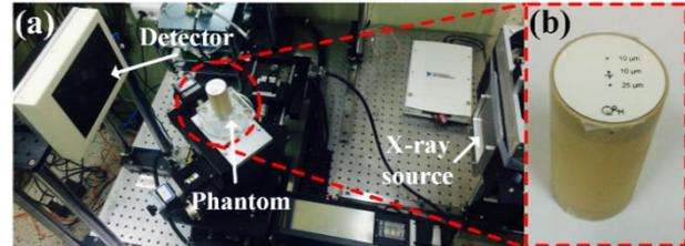
Fig. 1. The computed tomography system that was constituted for experiment (a), the thin wire phantom that was used in experiment (b).
