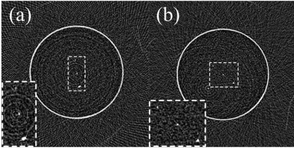
Fig. 2. Reconstructed tomographic image sample from continuous method (a), and step-and-shoot method (b). The wire tomography in the center of the image was enlarged.
