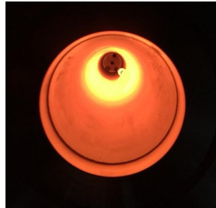
Fig. 5. Interior of furnace where specimen was installed (1200°C).
