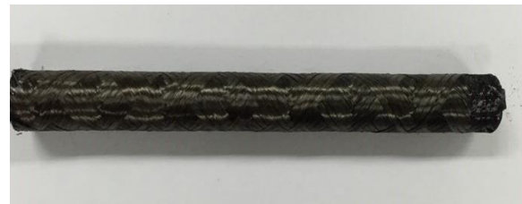
Fig. 1. SiC fiber preforms of SA3-S1I08PX helically wound with winding angle +55/-55° on Zircaloy-4.
