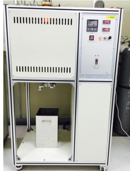
Fig. 4. Drop tube furnace for the thermal shock test.
