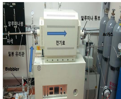
Fig 2. High-temperature discontinuous measurement oxidation equipment (tube furnace)
