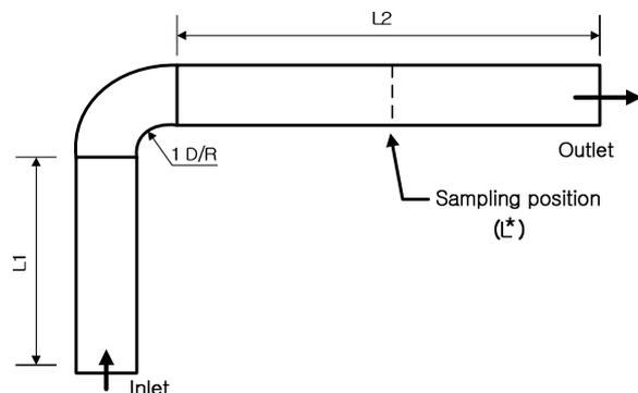
Figure 2.1 Analysis model with rectangular elbow duct
