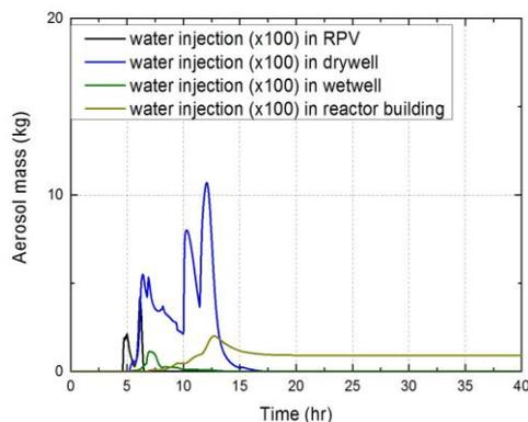
Fig. 4 Fission product behavior (a) base case (b) 100 times water injection case
