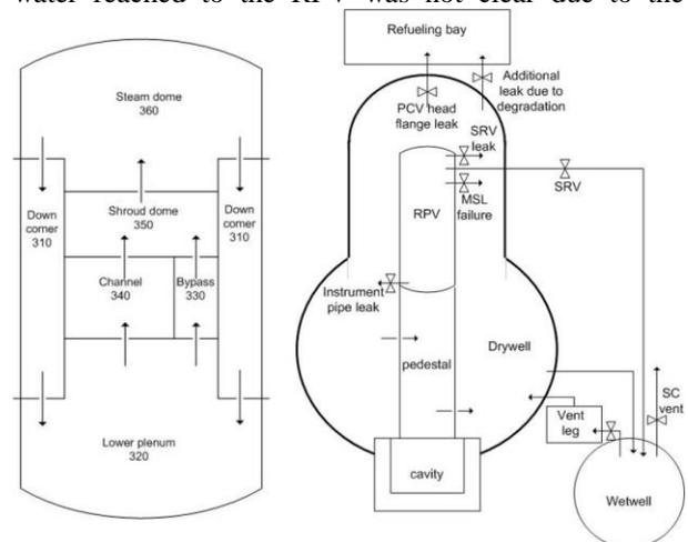
Fig. 1 Nodalization of RPV and PCV
