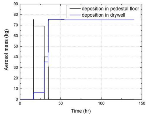
Fig. 6 Aerosol mass in deposition area in PCV (a) base case (b) 100 times water injection case
