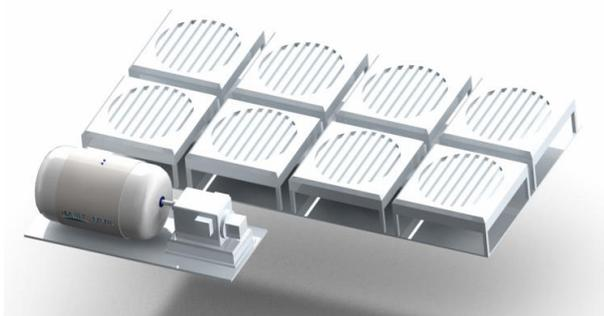
Fig. 6. Schematic of KAIST-MMR with CO<sub>2</sub> to air heat exchanger and synchronous generator (60Hz).
