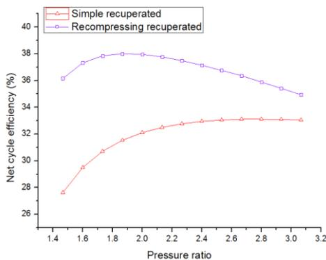
Fig. 5. Net cycle efficiencies of simple recuperated cycle and recompressing recuperated cycle with respect to pressure ratio.
