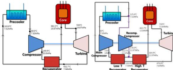
Fig. 4. Schematic figure of simple recuperated, and recompressing S-CO<sub>2</sub> Brayton cycle.
