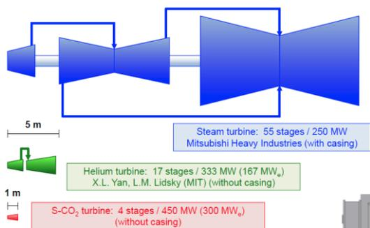
Fig. 1. Size of S-CO<sub>2</sub> turbine in comparison to the steam and helium turbine [1].
