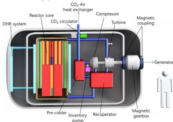
Fig. 2. Schematic figure of KAIST MMR.
