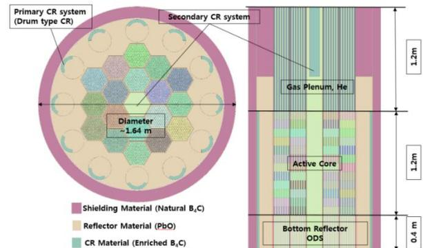
Fig. 3. Radial and axial configuration of the reactor core.
