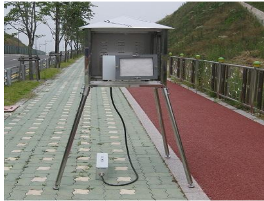
Fig. 1. Portable air sampler used for the collection of uranium particles
