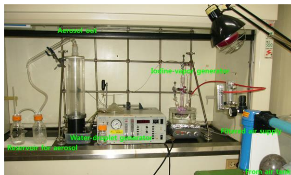
Figure 1: Photo of lab scale set-up for a behavioral study of volatile I 2 from water droplets - air flow.
