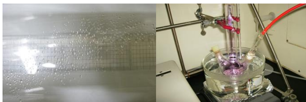
Figure 2: Monodisperse (48 \mu\text{m} size) water droplets produced by an aerosol generator (left photo) and volatile \text{I}_2 produced from solid \text{I}_2 by temperature controlling and air flowing (right photo).
