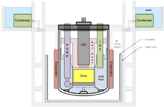
Fig. 1: Schematic diagram of ex-vessel thermosyphon
