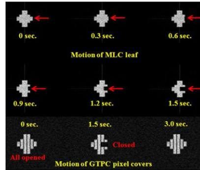
Fig. 2. Real time portal image of each collimator's moving pattern: (a) Multi-leaf collimator (MLC)'s leaf movement for 3.3 sec, and (b) Grid type multi-layer pixel collimator's (GTPC's) operation pattern for the same time.
