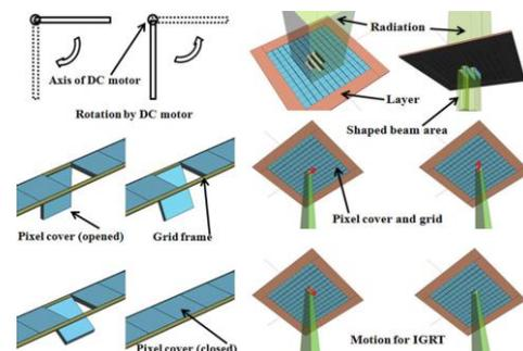
Fig. 1. The principle of the pixel cover operation. The blue cover could attenuate radiation regularly. General drawing of a grid type multi-layer pixel collimator (GTPC), showing open pixels to form the radiation beam's area and to partially attenuate the radiation and the pixel cover's movement for target guidance.
