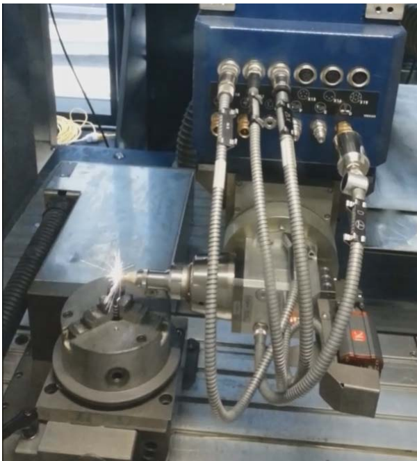
Fig. 5. Laser beam machining for the fabrication of tensile specimens from the unirradiated fuel cladding.
