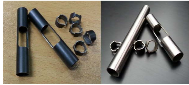
Fig. 6. Fabricated specimens from the unirradiated fuel claddings by using the laser beam machine for the tensile tests in longitudinal and hoop directions.
