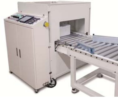
Fig. 1. Equipment of Technology for In-situation real time radioactivity inspection system.
