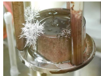
Fig. 2 U dendrite growth out of the LCC alumina crucible after the 7-hour deposition
