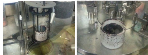
Fig. 4 Before (left) and after (right) the elimination of the salt in the LCC alumina crucible
