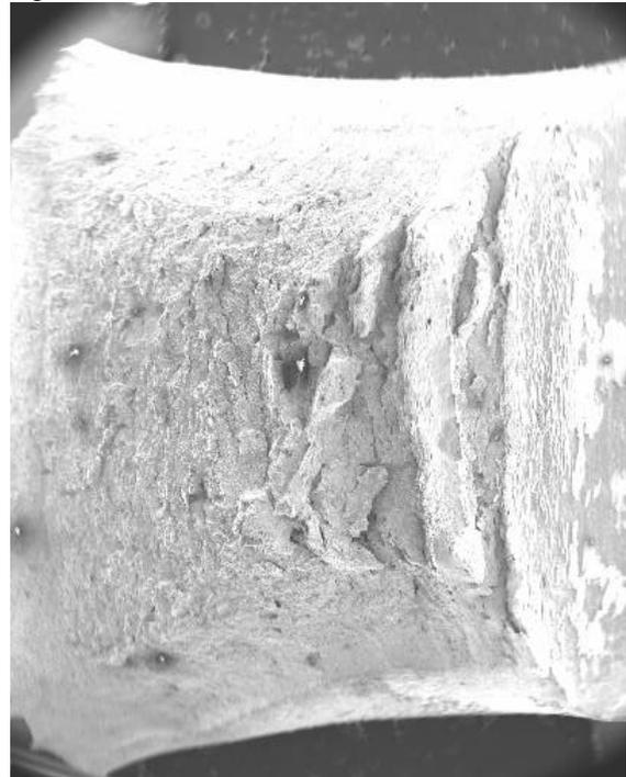
Fig. 3. Comparisons of fracture surfaces of SA 508 in a) as-received and b) aged at 400°C for 2,250H.
