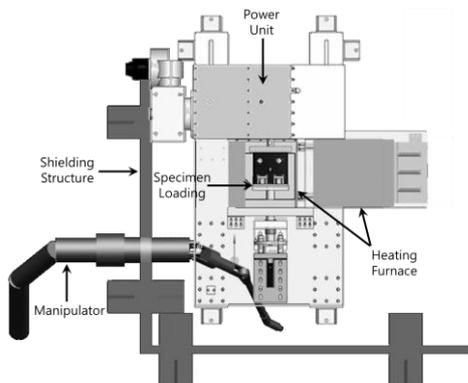
Fig. 1. Schematic of crush test system for irradiated spacer grid
