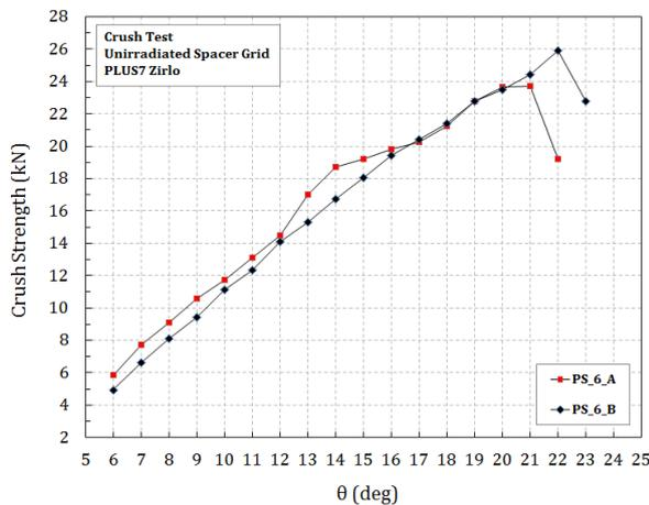
Fig. 3. Crush test results of un-irradiated PLUS7 mid spacer grid
