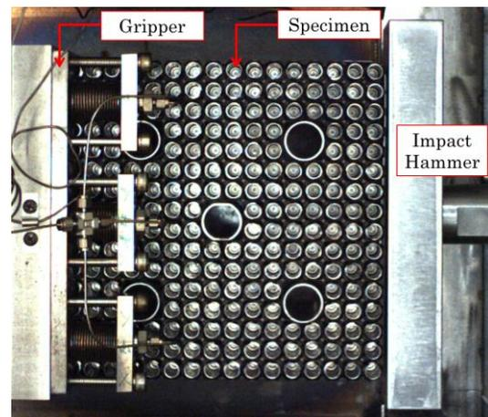
Fig. 2. Setting up of spacer grid for crush test
