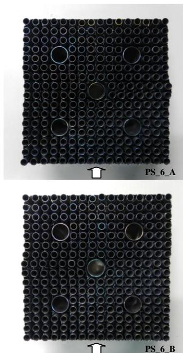
Fig. 4. Buckling mode shapes of un-irradiated PLUS7 mid-spacer grid by lateral impact load
