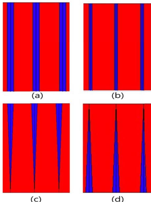
Fig. 2. Cross sectional views of the designed grids. (a) Thick parallel type, (b) Thin parallel type, (c) 'V' type, (d) 'Inverse V' type
