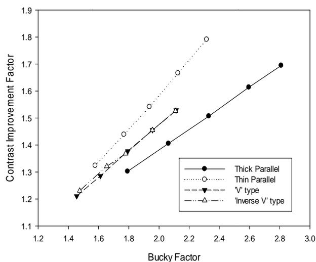
Fig 3. The contrast improvement factor according to the change of Bucky factor
