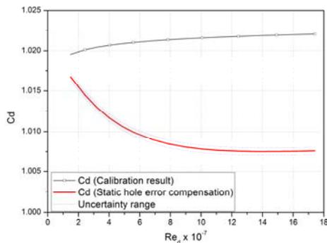
Fig. 3. Compensation of static hole error in discharge coefficient
