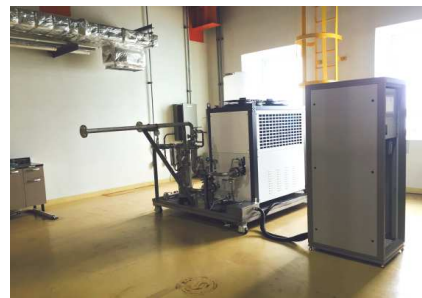
Fig. 9. Test Mock-up of target cooling system
