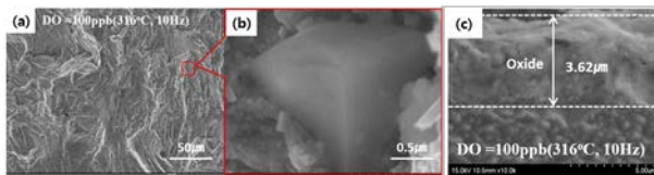
Fig.4. (a) Fatigue fracture surface, (b) its magnified image, and (c) its cross section image.
