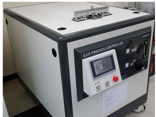
Fig. 1. The cold isostatic pressing equipment used for producing spherical matrix graphite samples
