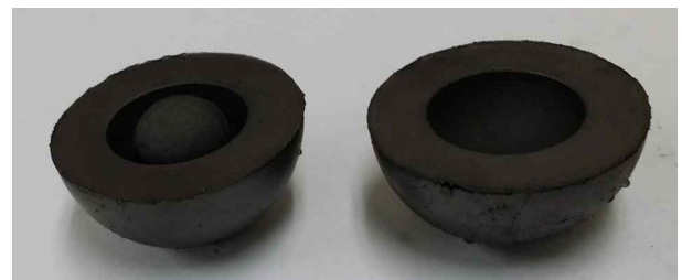
Fig. 2. A spherical graphite sample and the two semi-spherical mold after cold isostatic pressing
