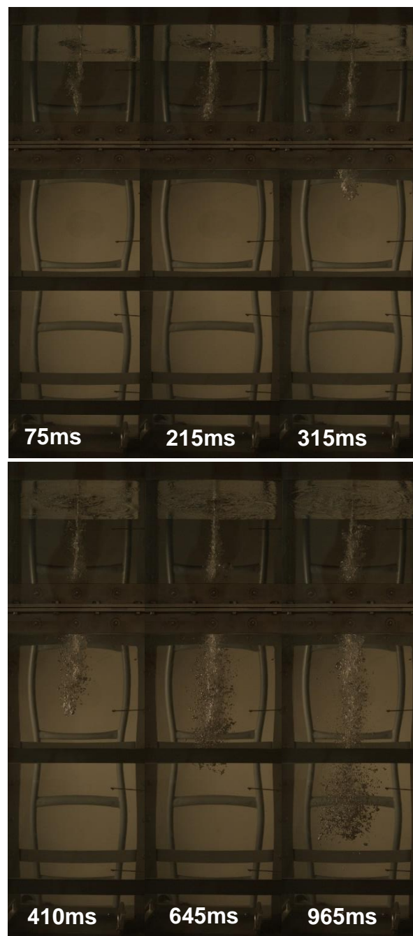
Fig. 4. High speed camera images (1920 \times 600, 1000 \mu s) with 14mm nozzle diameter
