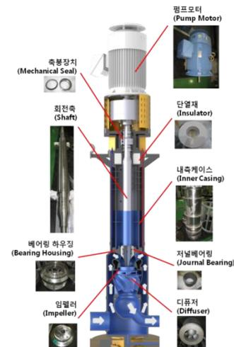
Fig. 1. Mechanical sodium pump
