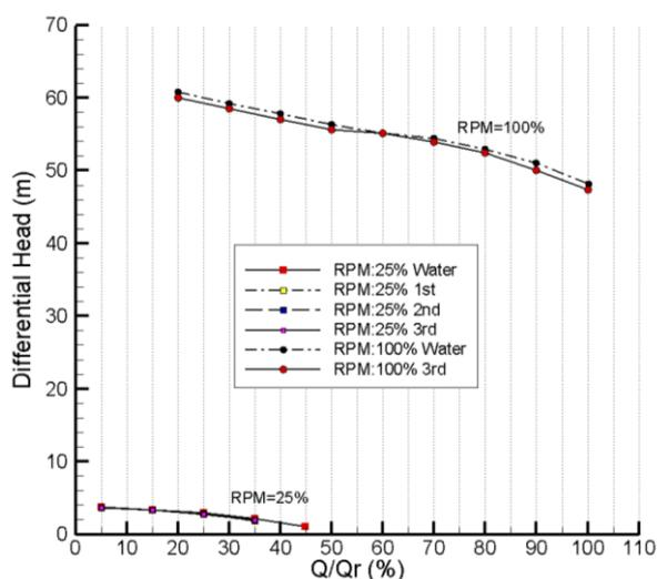
Fig. 6. The performance curve of 25% of rated RPM and rated RPM
