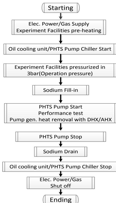
Fig. 4 The procedure of pump performance test,
