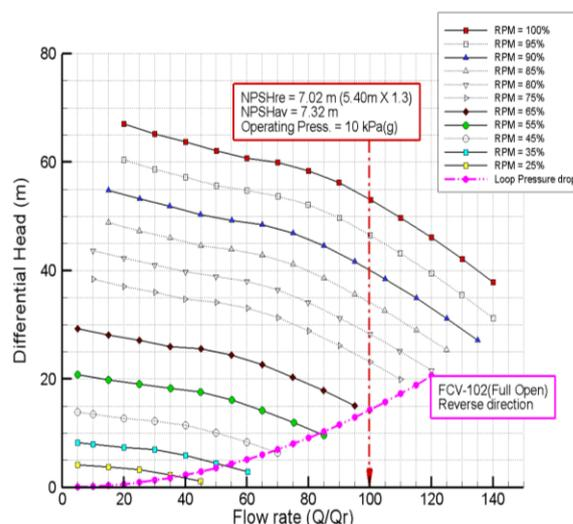
Fig. 7. The comparison between pump head with water environment experiment and pressure drop of test facility
