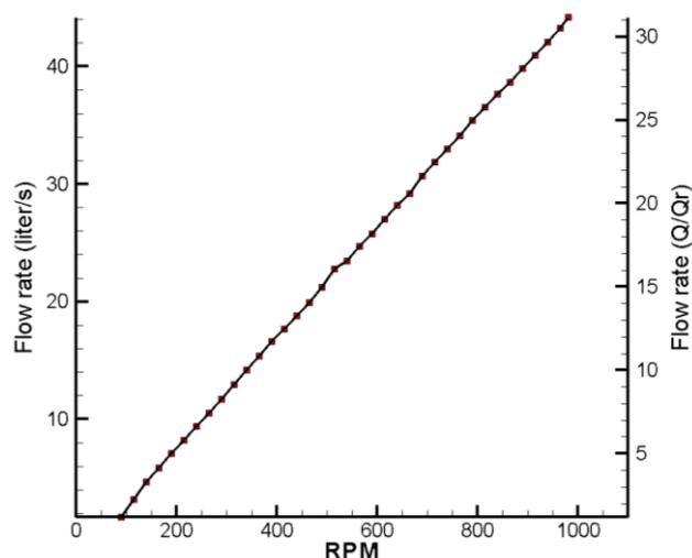
Fig. 5. The flow rate variation with RPM variation for 20% of opening rate of flow control valve
