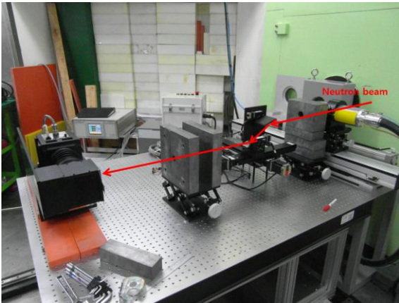
Fig. 3. The picture of the installed double crystal monochromator with imaging detector.
