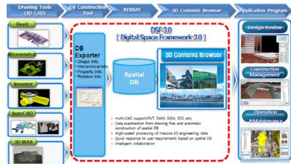
Fig. 2 FMS development Process based on BIM technology using Digital Space Framework 3.0
