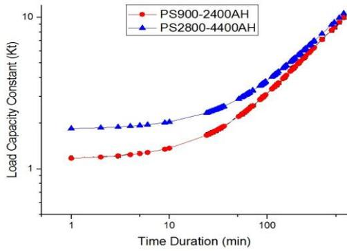
Fig.4. Log-Log curve to generate the  $K_t$  value based on eight hour.
