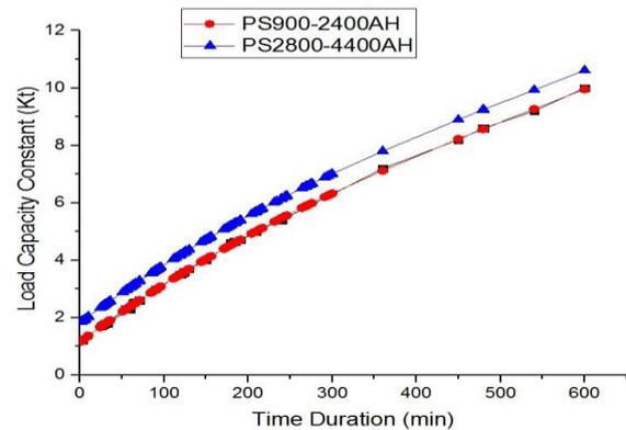
Fig.3. Discharge rate linear curve to generate the  $K_t$  value based on eight hour.
