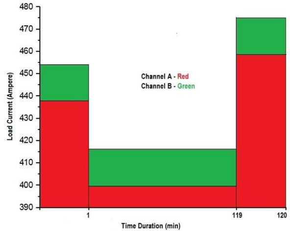
Fig.5. Duty cycle of load profile of channel A and B
