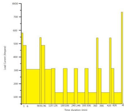
Fig.6. Duty cycle of the load profile on channel C battery of the NPP considered.
