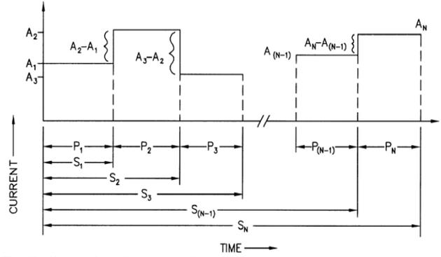
Fig.2. Generalized form of duty cycle.
