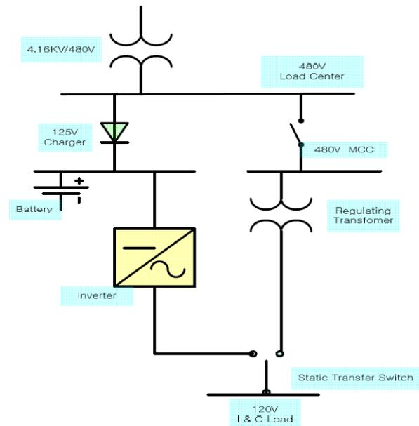
Fig.1. One of the trains of DC system of a nuclear power plant
