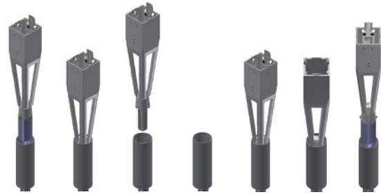
Fig. 2 Procedures for connection and disconnection between the ES adapter and the ES using a basket.
