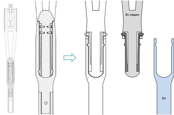
Fig. 1. Comparison of the geometry between the previous and the modified ESAs.
