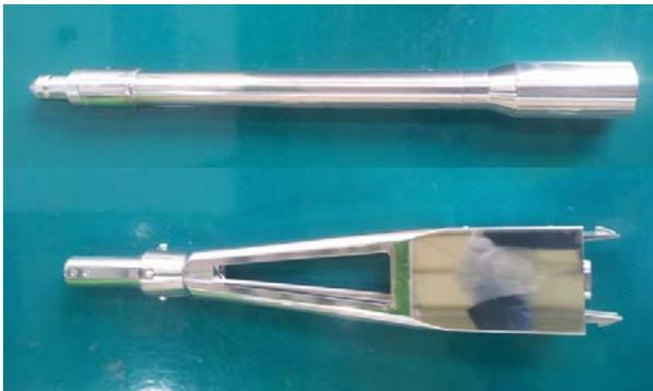
Fig. 7. Prototype of the ES adapter and shortened ES.
