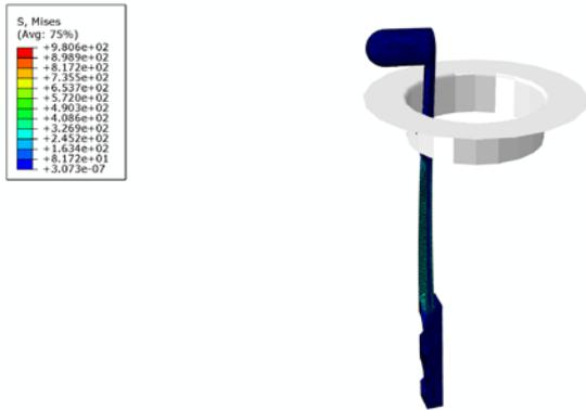
Fig. 6. Distribution of Mises stress at the maximum displacement from the contact analysis for the connection of the Inconel latch.
