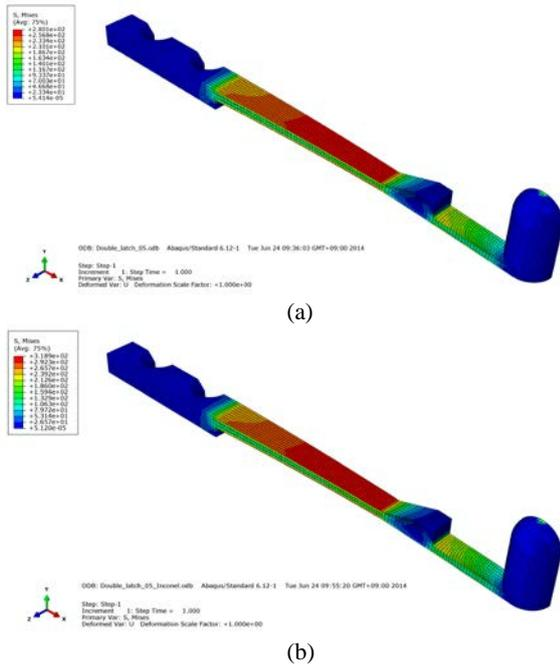
Fig. 3. Distribution of Mises stress at the maximum displacement 3 mm for (a) stainless steel and (b) Inconel latches.
