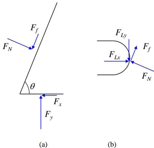
Fig. 4. Free body diagrams at the contact points of (a) the inclined basket and (b) the upper protrusion of the ES adapter latch.
