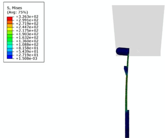
Fig. 5. Distribution of Mises stress at the maximum displacement from the contact analysis for the disconnection of the Inconel latch.
