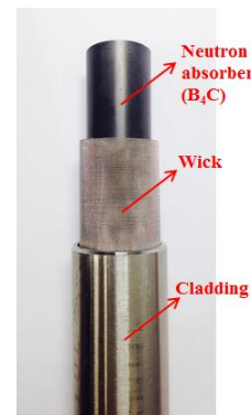
Fig. 1. Composition of hybrid control rod.
