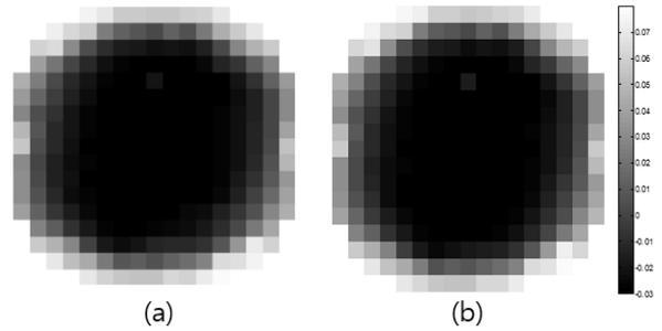
Fig. 5. Contour map of the core outlet pressure distribution (a: 4P-balanced, b:4P-balanced for intact LSS [4])
