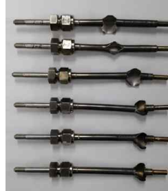
Fig. 5 Burst test result
