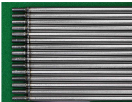
Fig. 2 weld specimens prepared by GTAW
