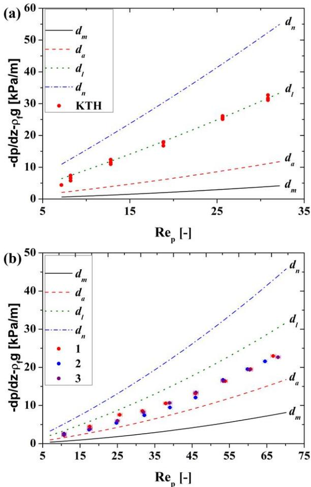
Fig. 5. Frictional pressure drops of water flow at  $Re_p > 7$  :
