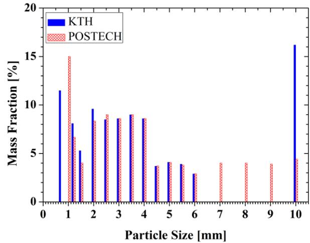
Fig. 6. Mass fractions of each particle size in Bed 5 of KTH and mixed bed of POSTECH.
