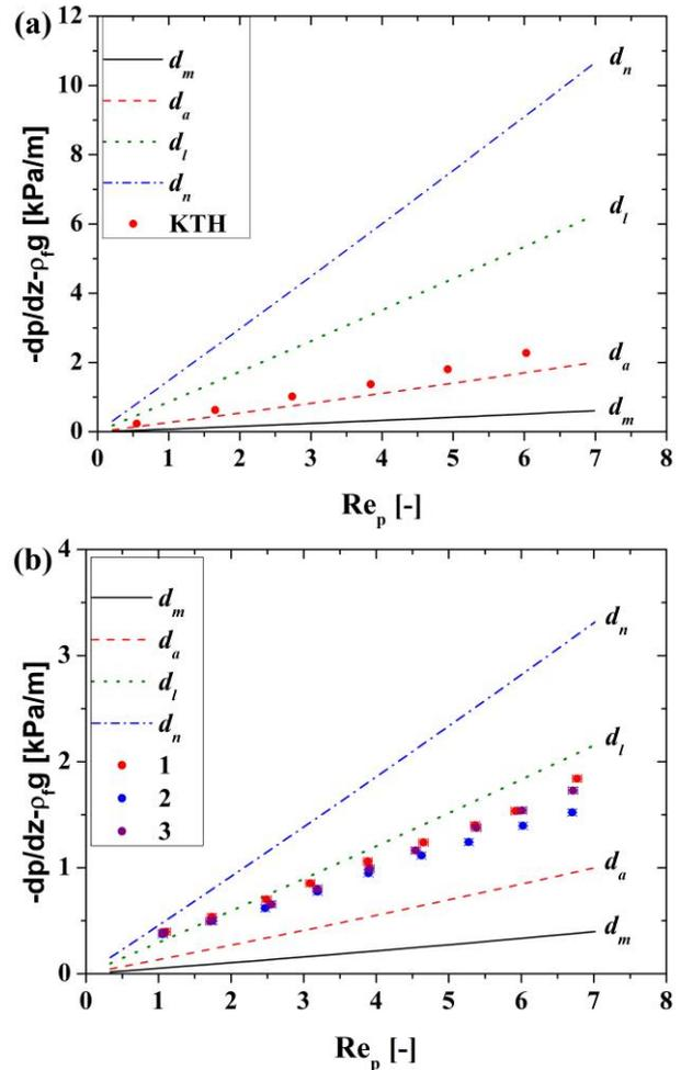
Fig. 4. Frictional pressure drops of water flow at  $Re_p < 7$  : (a) Bed 5 of KTH, (b) mixed bed in this study.
