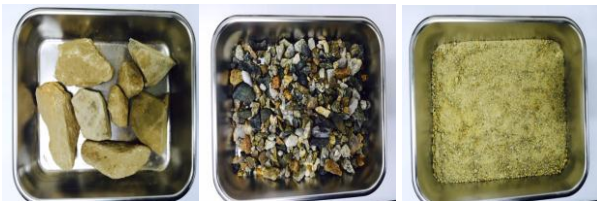
Fig. 1. Assortment of crushed gravel (initial state: left, after using a jaw crusher: middle, after using a pulverizer: right)
