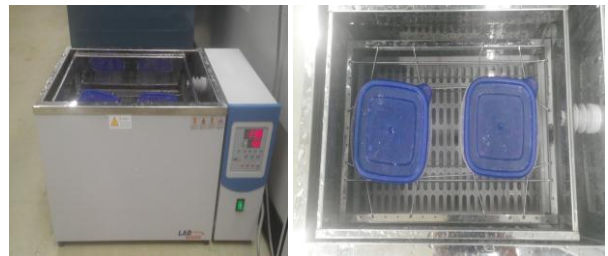
Fig. 2. Soil washing of U-contaminated gravel using a shaking incubator.
