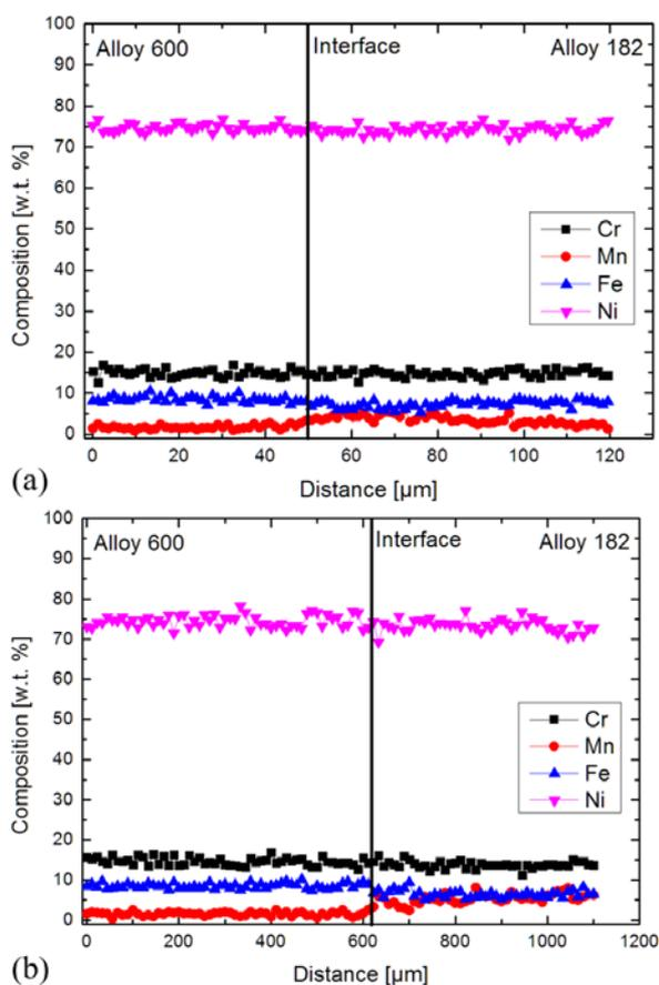
Figure. 7. EDS linear profile along the interface between Alloy 600 and Alloy 182 at (a) high magnification and (b) low magnification.
