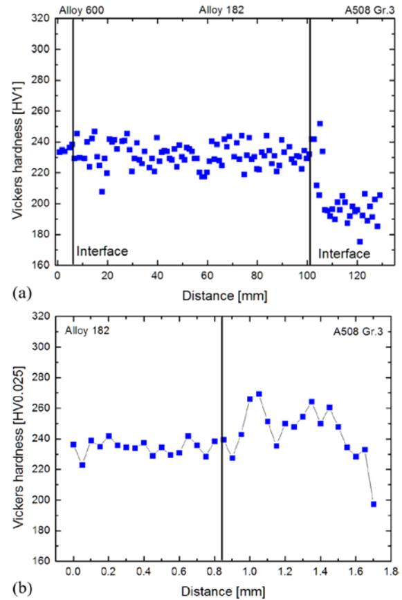
Figure. 3. Distribution of Vickers hardness on (a) whole range of DMW, (b) narrow range at the interface between Alloy 182 and A508 Gr.3
