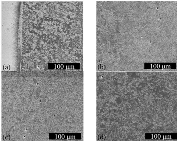
Figure 4. Microstructures of A508 Gr. 3 which have (a) coarse-grained HAZ, (b) fine-grained HAZ, (c) intercritical HAZ, and (d) subcritical HAZ structure respectively
