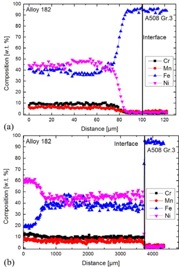
Figure 6. EDS linear profile along the interface between Alloy 182 and A508 Gr. 3 at (a) high magnification and (b) low magnification.
