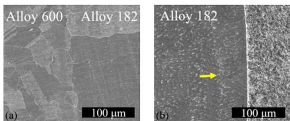
Figure 5. Microstructure of (a) the interface between Alloy 600 and Alloy 182 weld metal, (b) the interface between Alloy 182 and A508 Gr.3 weld metal. The yellow arrowed line is Type-II boundaries.
