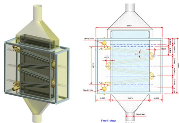
Fig. 4. The details of M-FHX including a front-view.
