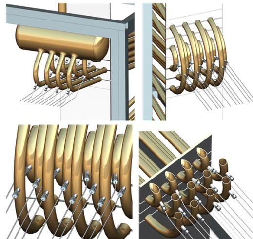
Fig. 3. The schematic drawings of the instrumentation to measure sodium temperature inside every tubes.
