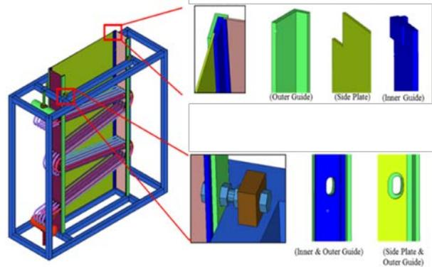
Fig. 2. The conceptual design of flow guide plates of M-FHX to allow the thermal expansions of each plate.
