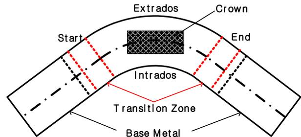
**Fig. 1** Locations of specimens used for the experiment in SA312 TP347 pipe bend
