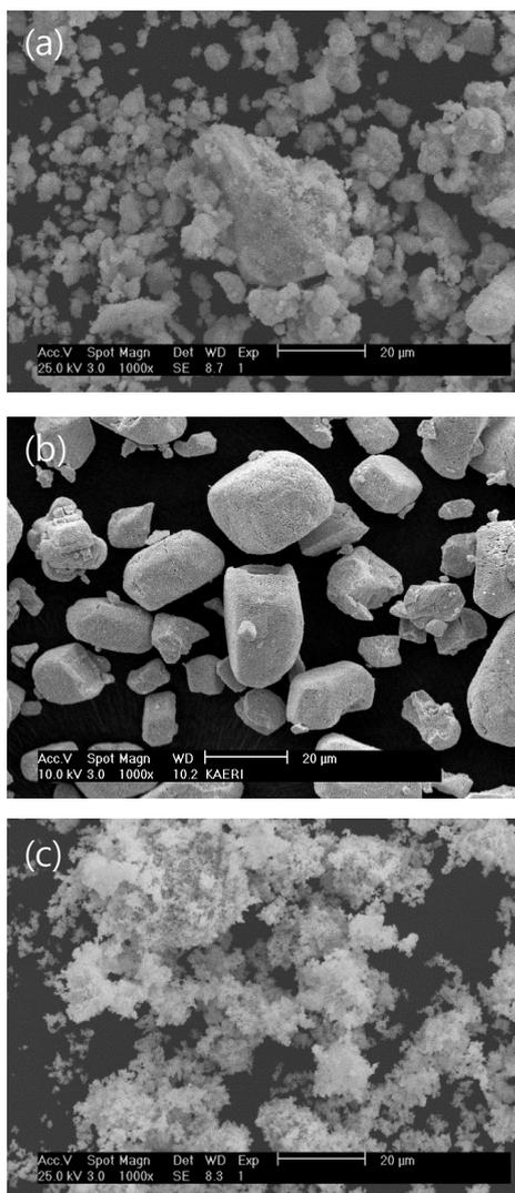
Fig. 2. SEM images of the different routes of UO<sub>2</sub> powders; (a) ADU-UO<sub>2</sub>, (b) AUC-UO<sub>2</sub>, and (c) IDR-UO<sub>2</sub>.
