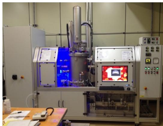
Fig. 1. Thermo-optical measurement system, TOM-AC.
