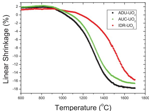
Fig. 3. Sintering Shrinkage of UO<sub>2</sub> compacts from the different powder routes.
